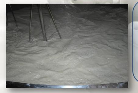
The initial milk acidity, the temperature, the quantity of rennet used, the enzymatic composition of the rennet and the protein contents of the milk are usually the main factors that influence the coagulation process.
