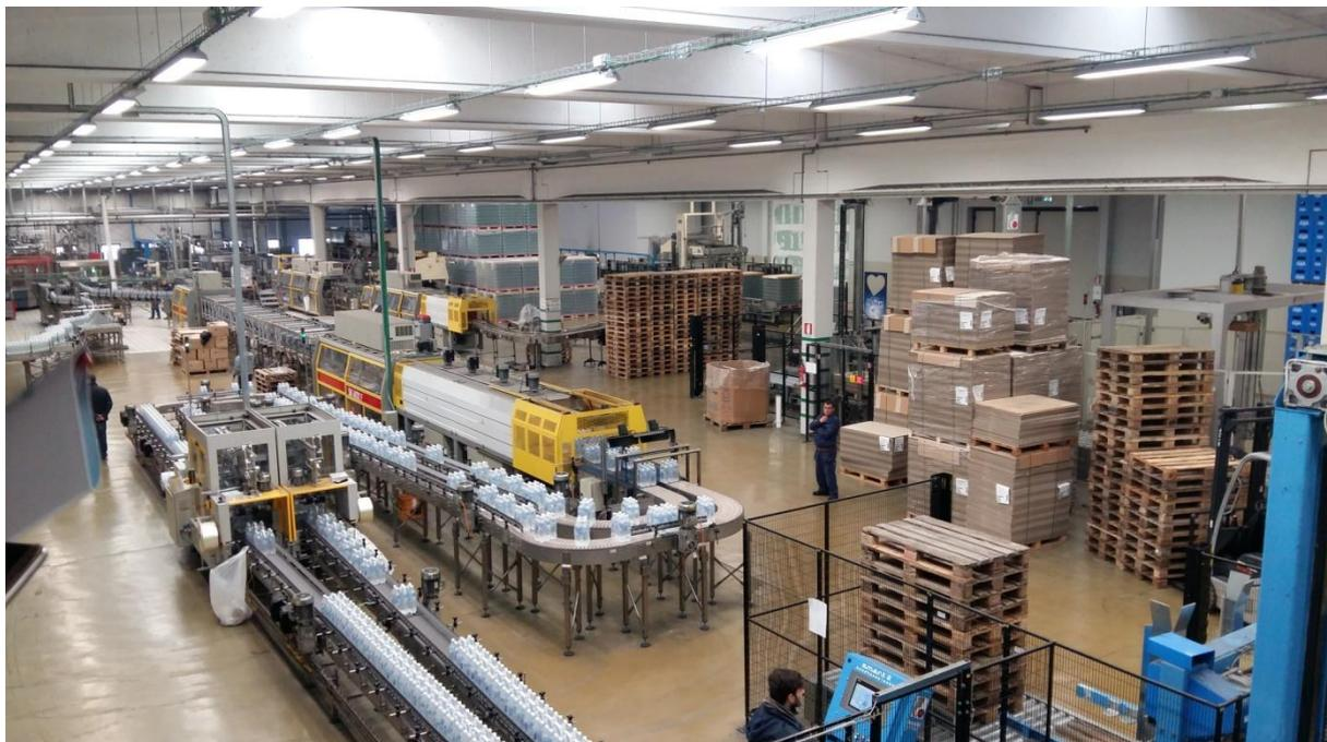
Here's the main hall with some of the machinery used for the production of Di Iorio's products. The factory has two bottling lines: PET line for plastic bottles and Glass line
