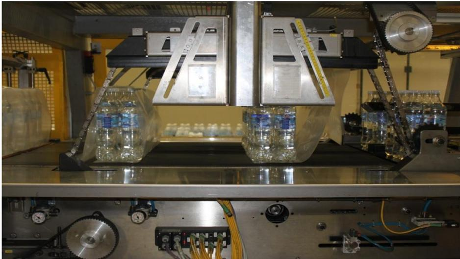
Filled bottles are packed with an heat-shrinkable plastic sheet
