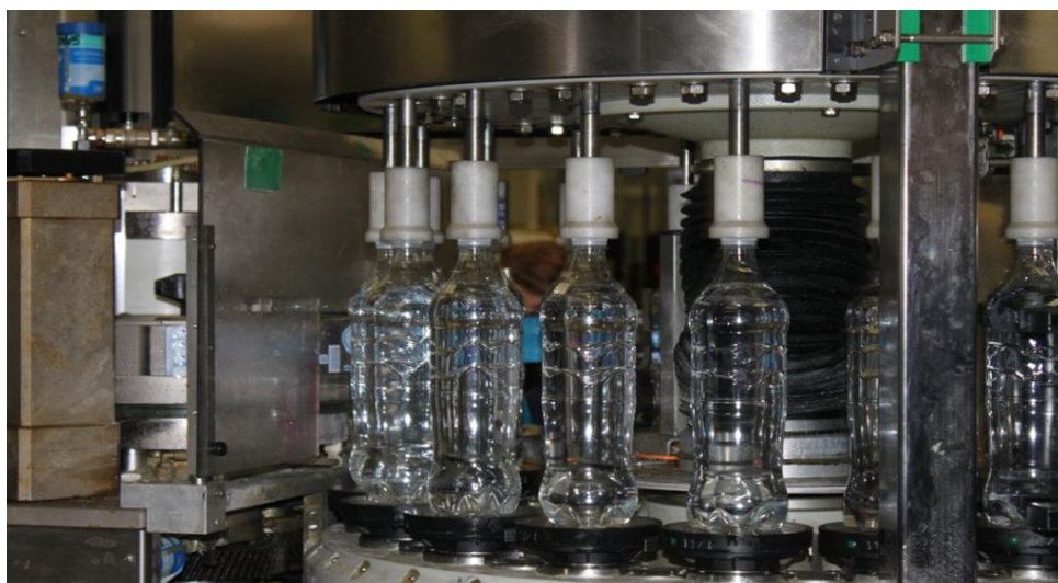
Then hot preforms are inflated with air to create Molisia bottles
