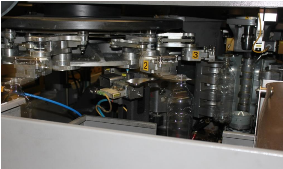
Then hot preforms are inflated with air to create Molisia bottles
