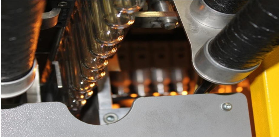
This is the first step of the production. These small plastic pipes called “preforms” are heated in an oven.
